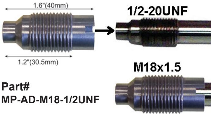
MPI - M18x1.5 to 1/2"-20UNF adaptors can be used as an emergency replacement to convert a stock 1/2"-20UNF transducer/transmitter to fit in a M18x1.5 non-stock pressure port.
